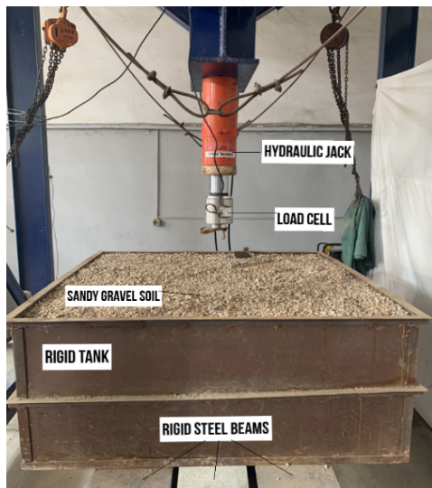
Fig. 2. Test Tank Configuration for Soil Layer Boundaries.
